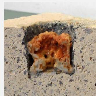
Refractory NOT attacked by alkali
